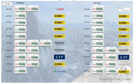
Additional programming will be engineered to allow visual and emailed alarms of energy over usage and out of hours use allow maintenance to be proactive on energy saving.
